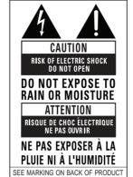
THE LIGHTNING FLASH AND ARROWHEAD WITHIN THE TRIANGLE IS A WARNING SIGN ALERTING YOU OF "DANGEROUS VOLTAGE" INSIDE THE PRODUCT.
